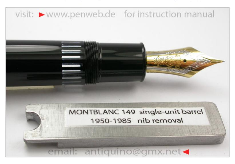
You can see the nib carrier and the two notches (slots) inside the nib unit. The slots must be exactly in 12 and 6 o`clock position below and above the nib. This is the original position. If the slots are not in the right position you cannot go further without damaging the nib as well as the feed!
